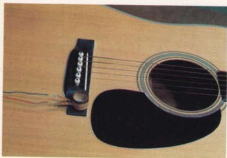
*Transducer mounted on bridge*
