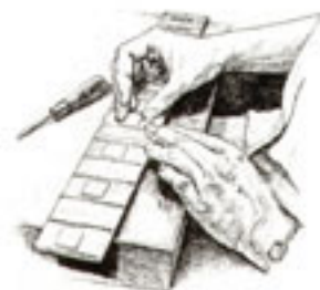
Installation of fingerboard inlays
