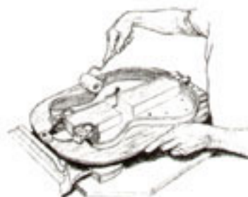
Hand application of top & bottom to rims
