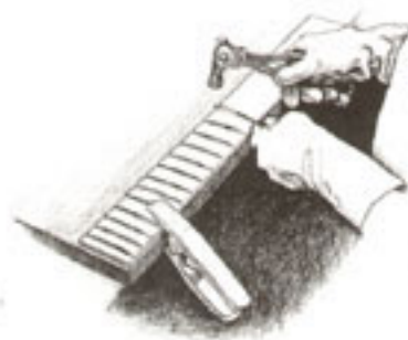
Installation of frets into neck
