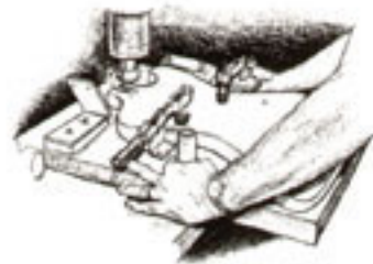
Routing solid body for neckpiece
