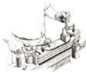
Hand guiding through router in shaping the neck
