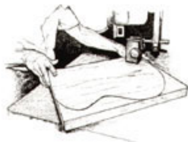
Band saw cutting body shape
