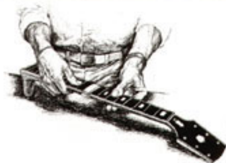
Fret board positioning and installation
