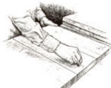
Matching wood panels for grain and color
